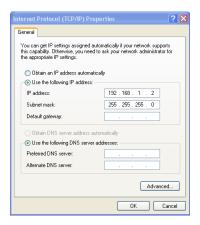
Figure 7: Internet Protocol (TCP/IP) Properties Window
